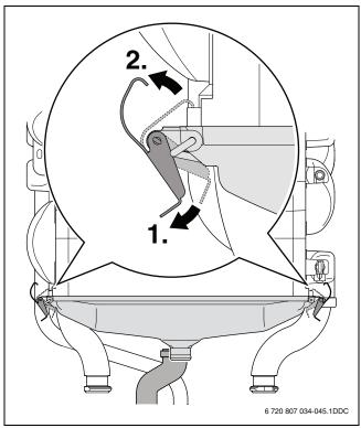
Fig. 64 Opening the snap fasteners of the condensation catch pan
