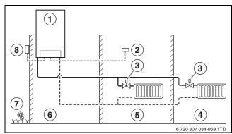
Fig. 25 Principle of weather-compensated control
