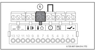
Fig. 34 Connecting the outside temperature sensor
