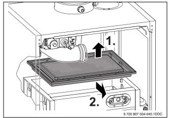
Fig. 57 Removing the burner
