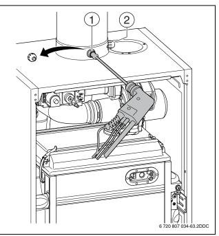
Fig. 48 Removing the cap of the flue gas testing point.
