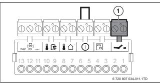
Fig. 31 Connecting the on/off room temperature-dependent control unit
