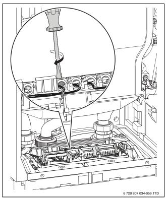
Fig. 30 Tightening the screw
