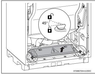
Fig. 27 Removing the cover
