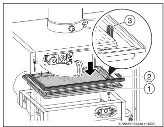
Fig. 61 Inserting the burner with gasket
