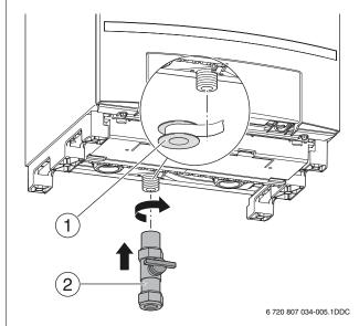
Fig. 15 Installing the gas isolator
