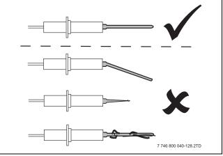
Fig. 59 Checking the monitoring electrode
