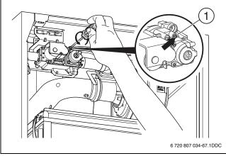
Fig. 46 Open the burner pressure nipple at the type 70
