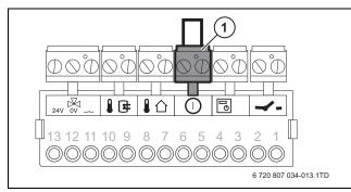
*Fig. 33* Connection of an external switching contact
