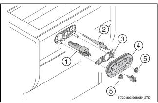
Fig. 60 Replacing the ignition device
