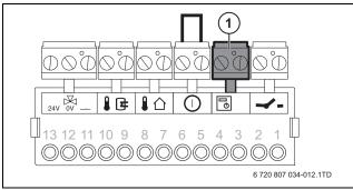
Fig. 32 Connection of the modulating controller
