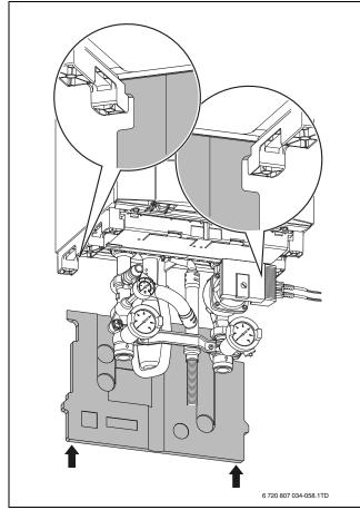
Fig. 22 Mounting the back panel (insulation)
