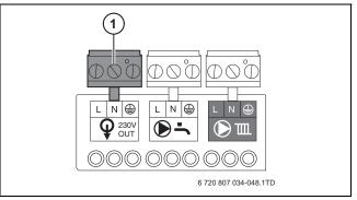
Fig. 35 Connecting the mains voltage
