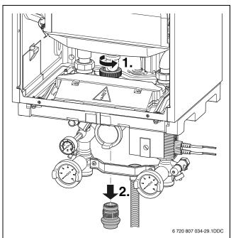
Fig. 18 Remove the transport protection
