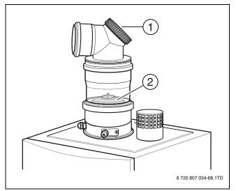
Fig. 70 Checking the flue gas pressure-relief valve
