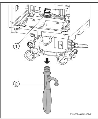
Fig. 62 Removing the condensate trap
