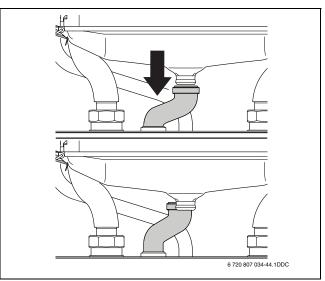
Fig. 63 Remove the condensate hose
