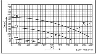
Fig. 7 Residual head per type, with connection set and non-return valve
