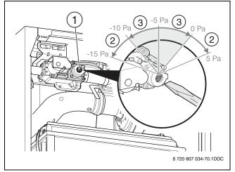
Fig. 68 Setting the gas/air ratio at the Type 70
