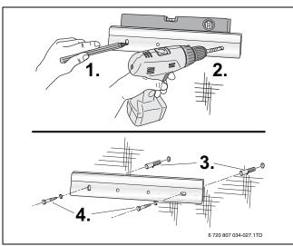
Fig. 10 Installing the mounting rail on the wall
