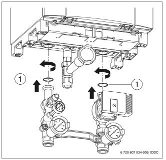
Fig. 14 Mounting the connection set
