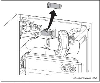
Fig. 52 Removing the gas supply pipe
