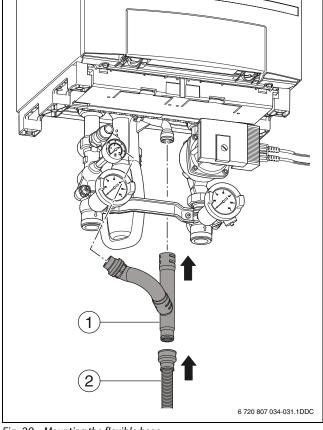
Fig. 20 Mounting the flexible hose
