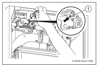
Fig. 42 Open the burner pressure nipple at the type 70
