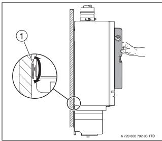
Fig. 11 Aligning the gas condensing boiler
