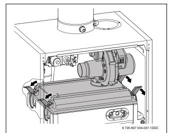
*Fig. 54 Opening the snap fasteners*
