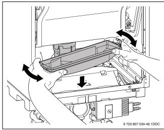
Fig. 65 Removing the condensate pan
