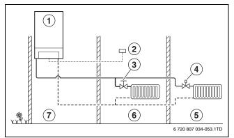
Fig. 24 Control principle of room temperature-dependent control
