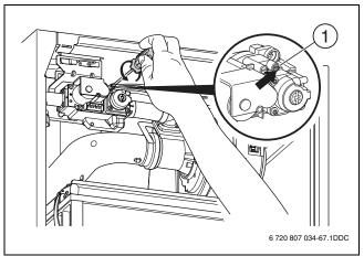
Fig. 66 Opening the burner pressure test nipple at Type 70
