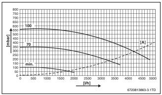
Fig. 8 Residual head per type, with connection set
