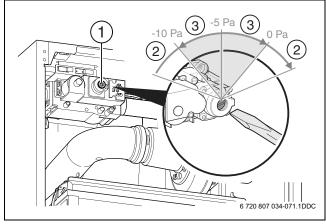
Fig. 69 Setting the gas/air ratio at the Type 100
