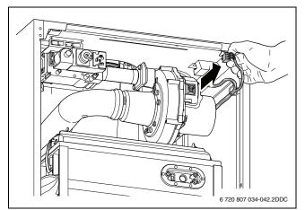
Fig. 51 Removing the mains plug of the fan
