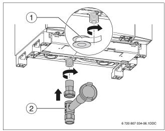
Fig. 13 Installing the gas isolator
