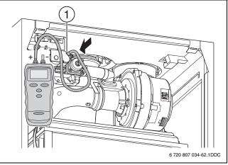
Fig. 44 Connecting the pressure gauge at type 70
