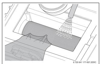
Fig. 58 Cleaning the heat exchanger
