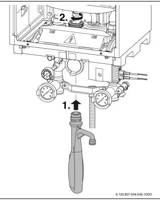
Fig. 19 Installing the condensate trap
