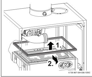
Fig. 56 Removing the burner gasket
