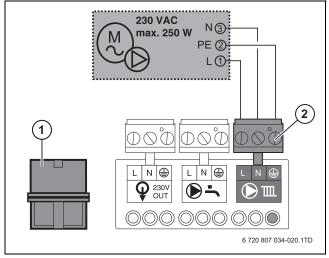
Fig. 36 Connection of pump
