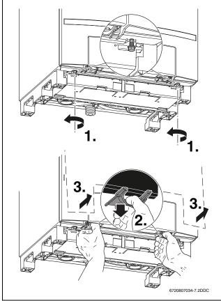
Fig. 2 Casing removal
