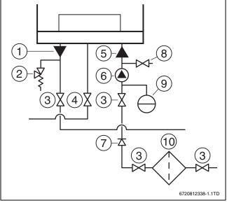
Fig. 16 Connection of the heating water pipework
