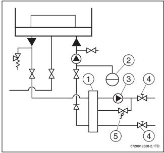
Fig. 17 Installation of the low loss header
