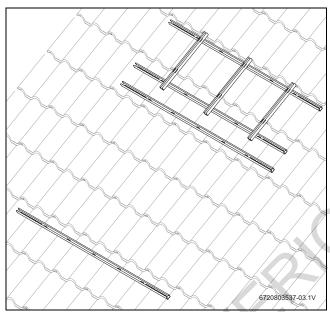
Fig. 21 Pre-assembled profile rails for two collectors
